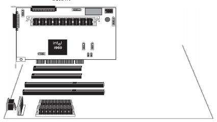
Screw the bracket to the computer frame.
